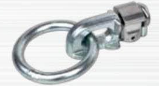
6072-O Double stud fitting with Round Ring, 2727kgs/6000lbs
