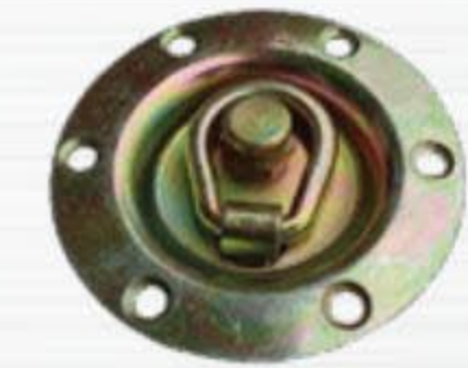
PPE-14 Recessed Rotating Rope Ring-Bolt on or Weld-on, 1360kgs/3000lbs
