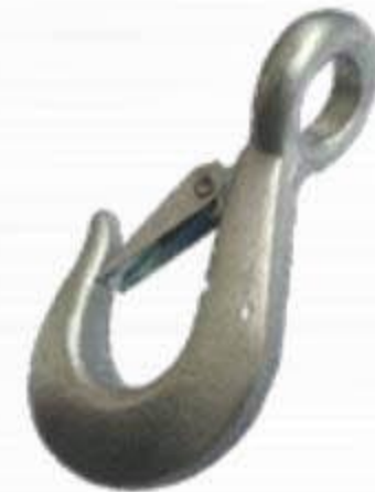
HK-14 Forged Eye Twisted Hook, 3500kgs/7700lbs
